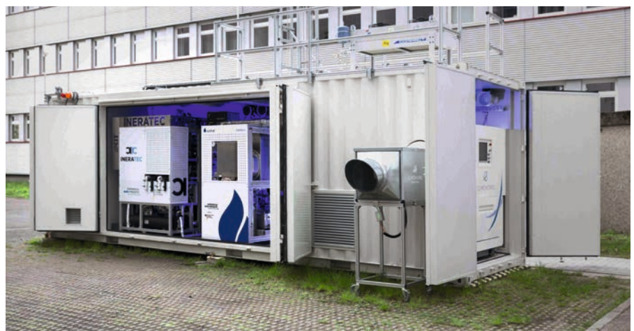
All four process stages involving the partner entities Climeworks, Sunfire, Ineratec and Kit are brought together in a single system in this container.
