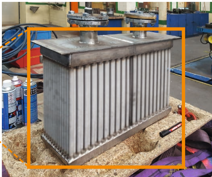
New high-performance recuperator: same level of performance, 25 times smaller in size.
