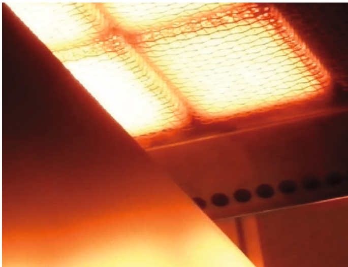
Steel belt dryer with porous burner, offering a higher energy density and accelerating heat transfer into the conveyor material without impairing product quality.
