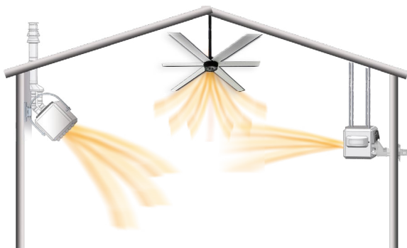
Example 1: warm air heater mounted at the wall with horizontal warm air outlet, with an additional ceiling fan.
