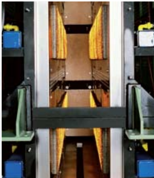
A look inside a gas infrared pre-dryer without a web
