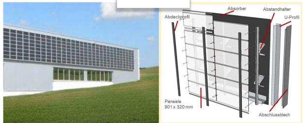
>> GOGAS – LUBI WALL – ALWAYS FRESH AND FILTERED AIR – 30% GRANTS FRESH AIR SOLAR COLLECTOR – AEROSOLE INFECTIONS
